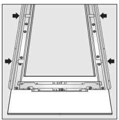
Insert the angle trim (15) as far as it will go into the spaces in the frame, as shown.
